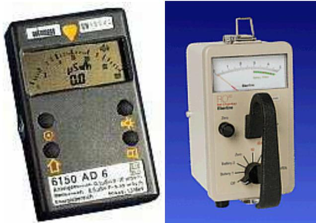
Figure 3. Examples of survey meters - they measure exposure rate.
