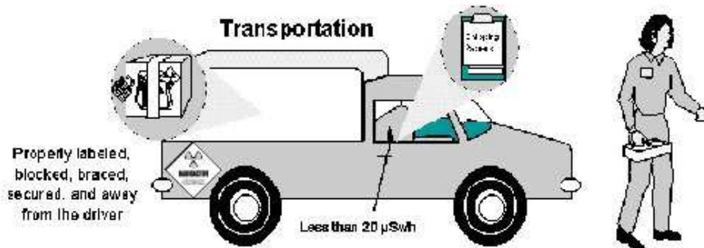
Figure 4. Basic requirements for transportation of sources.
