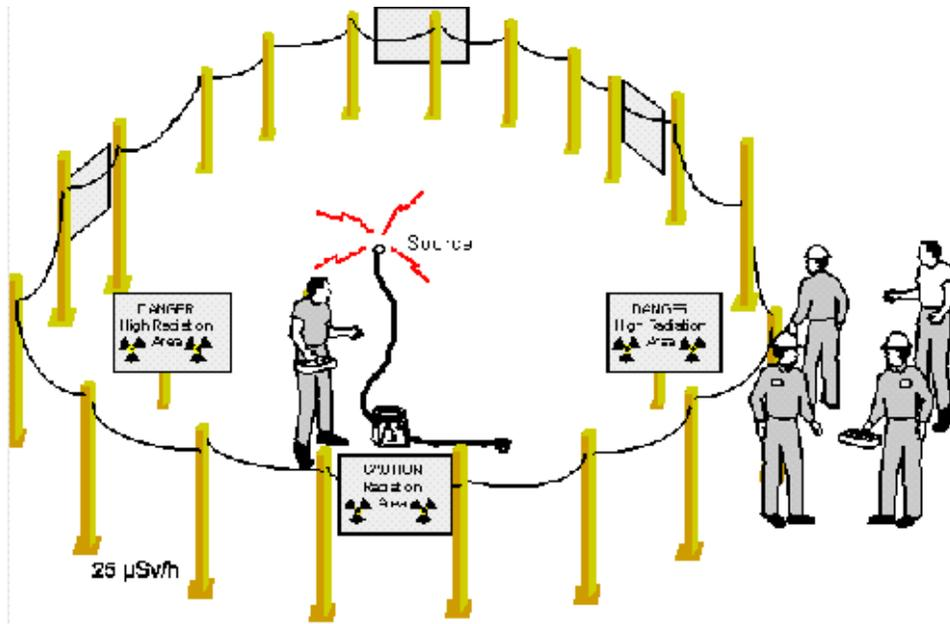
Figure 5. The dose rate at the barriers of a field site must not exceed 25 µSv/h.
