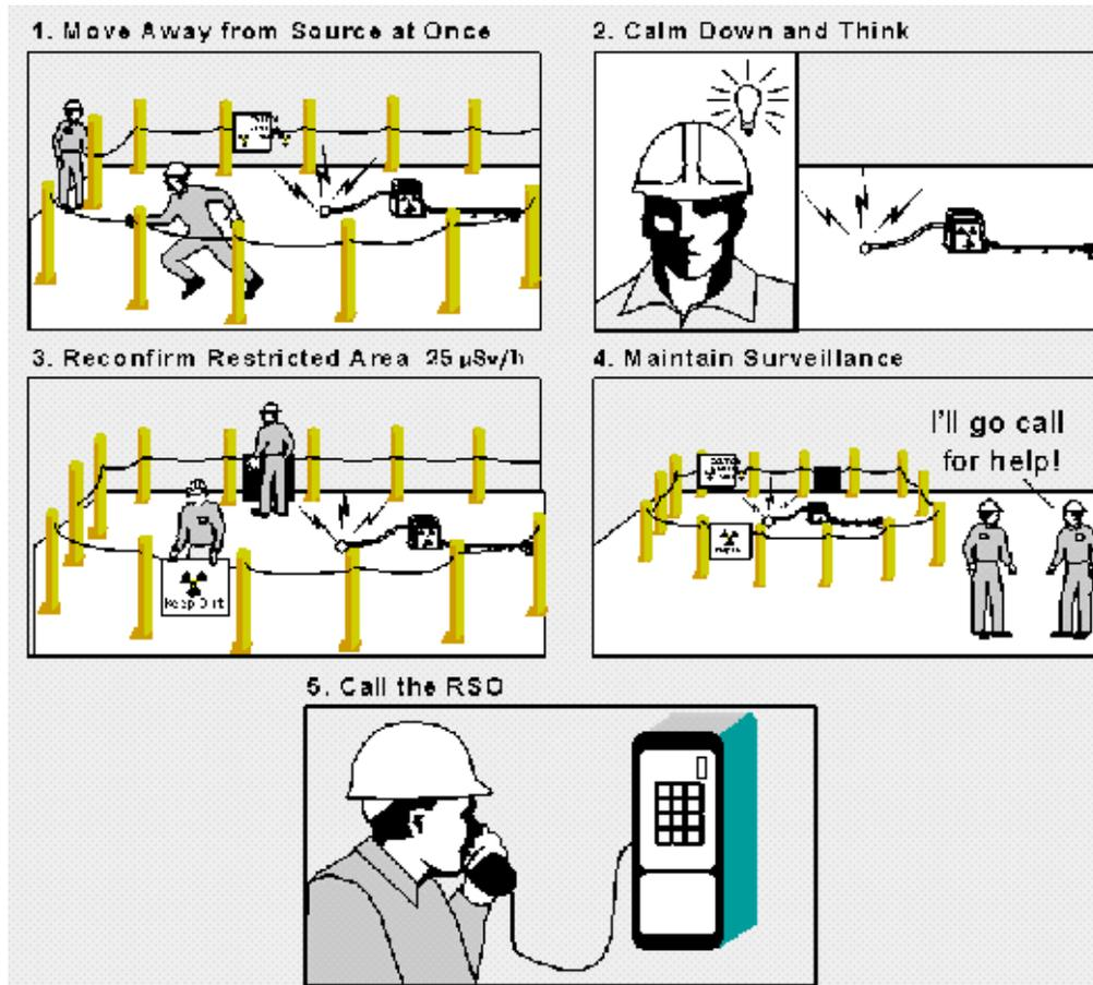
Figure 7. The registrant must have formulated emergency procedures and working rules. A copy of which should be available to all workers using industrial radiography equipment.
